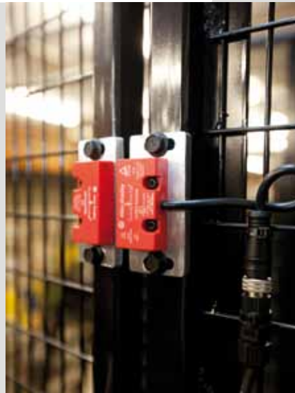
Interlock Guard Sensor
